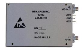
**AKON** has developed a new series of DLVAs operating over a frequency range of 0.5 to 18 GHz in a variety of bands. This new series offers 70 dB dynamic logging range with linearity of +/-1 dB over this range.
